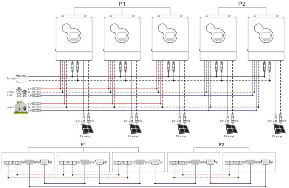
**e) Six all-in-one solar charger inverters of the system connected in two phase:**
