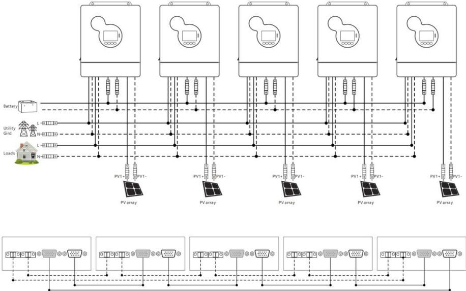
**e) Six all-in-one solar charger inverters of the system connected in parallel:**
