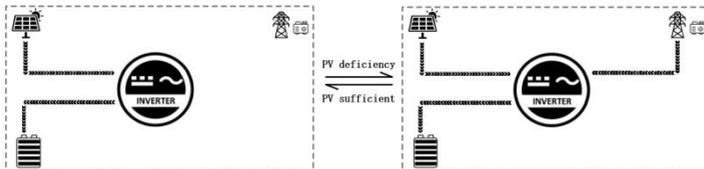
**4、 Only Solar:** Only PV charging, no mains charging is initiated. This is the most energy-efficient mode and the battery power comes from solar energy, which is usually used in regions with good daylighting conditions.
