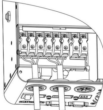
**Note:** The grounding wire shall be as thick as possible (cross-sectional area is not less than  $4\text{mm}^2$ ). The grounding point shall be as close as possible to the all-in-one solar storage inverter. The shorter the grounding wire, the better.
