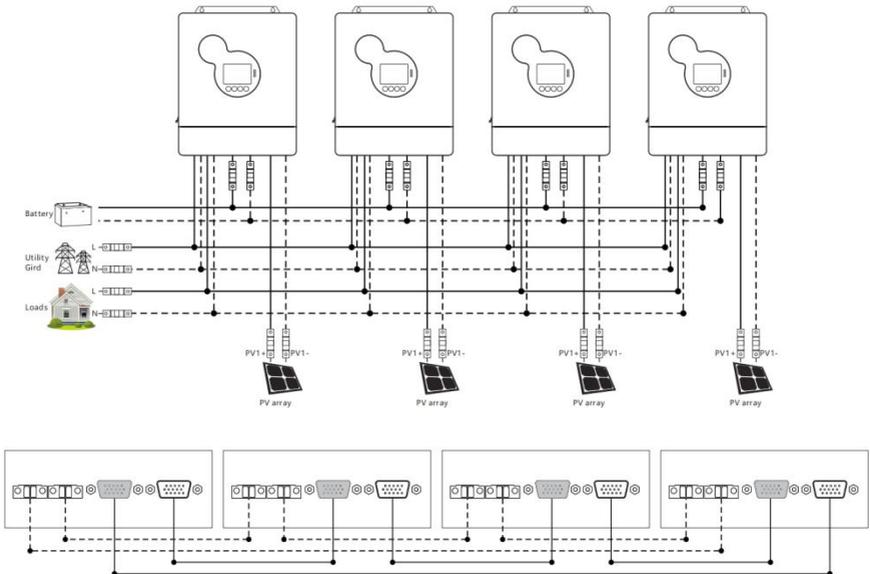
**d) Five all-in-one solar charger inverters of the system connected in parallel:**
