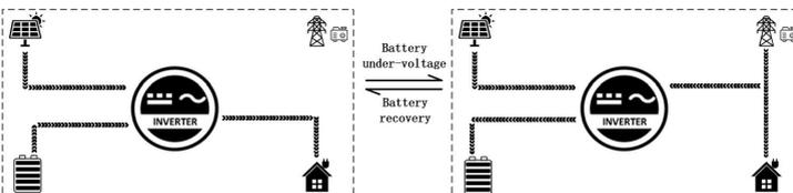
**4、Hybrid output and grid connection ( need to be abled)** In the utility bypass state, when no battery is connected or when the battery is full, the load power is supplied by the PV and the utility together if the hybrid function is enabled, and the surplus PV energy is fed back to the grid if the grid connection function is enabled.
