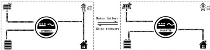
**3、 Inverter First:** switch to Mains Power supply only when the battery is under-voltage. This mode uses DC energy to the maximum extent and is used in regions with stable power grid.
